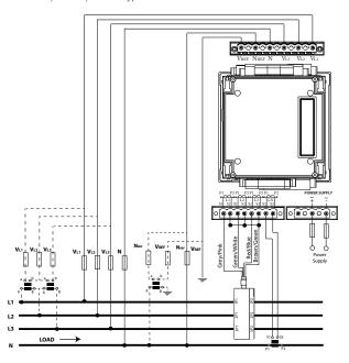
Direct phase-phase measurement with current transformers
