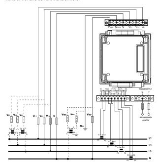
Three-phase measuring with or without voltage transformer and MC3 (250 mA) + MC1 type transformers for neutral current.
